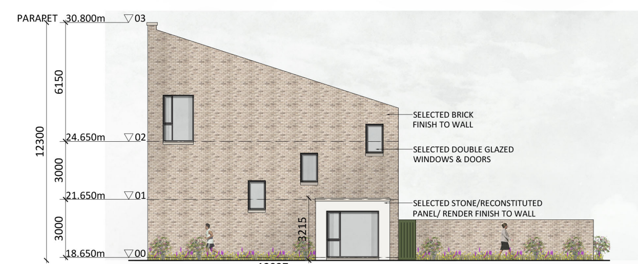
PKS DUPLEX END TERRACE (RIGHT) SIDE ELEVATION 1:200
