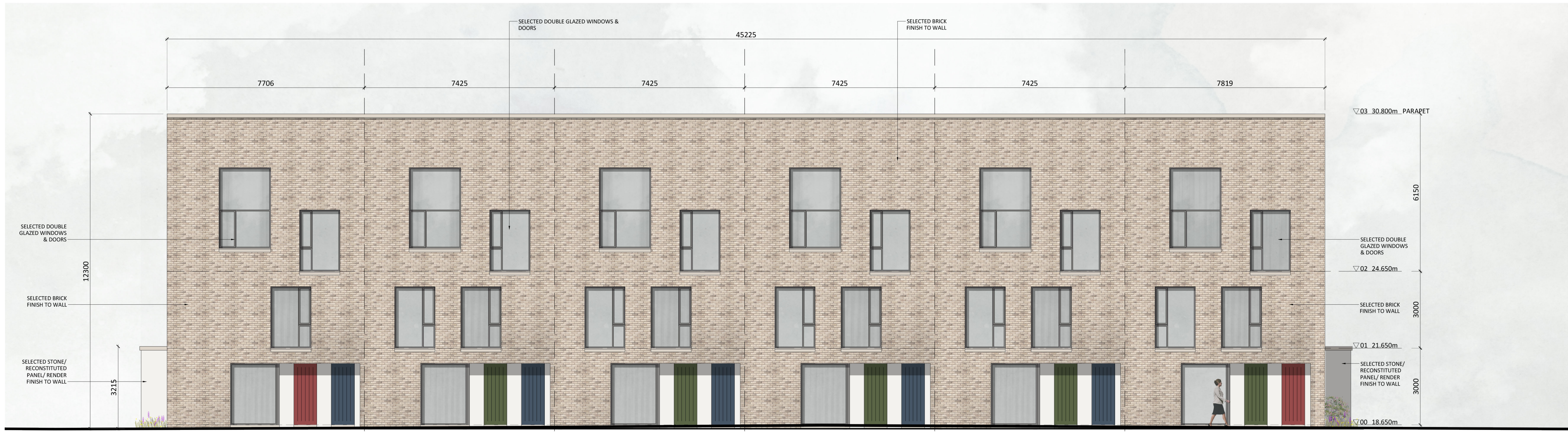
PKS DUPLEX TERRACE FRONT ELEVATION 1:100
