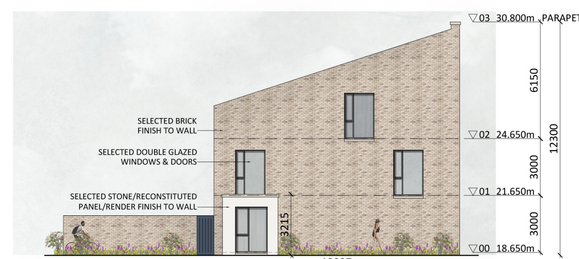
PKS DUPLEX END TERRACE (LEFT) SIDE ELEVATION 1:200
